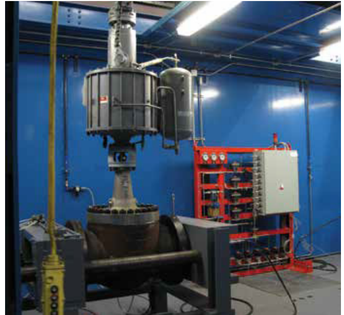
Gas testing and certification to the latest industry standards is performed by independent inspectors.
